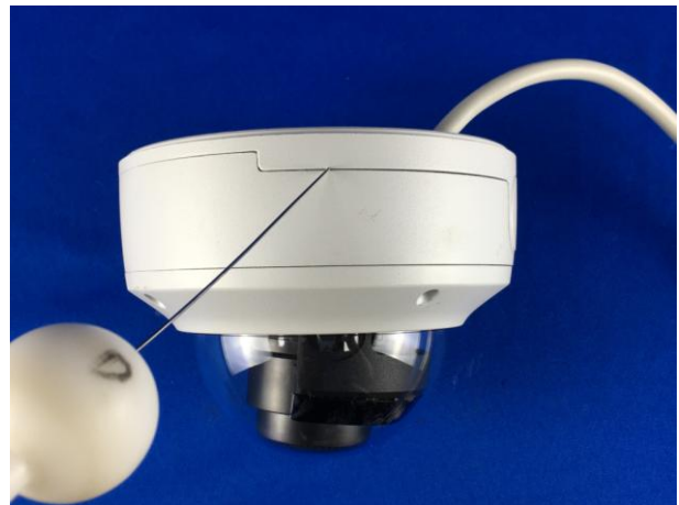
The 1.0mm test stick can not enter the gap of the sample
