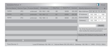
③ Modify the IP address. The default IP address of this camera is 192.168.1.168. Click the information of the camera listed in the above table to show the network information on the right hand. Modify the IP address and gateway of the camera and make sure its network address is in the same local network segment as that of the computer. Please modify the IP address of your device according to the practical situation.
