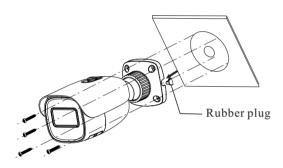
④ Bracket adjustment. Before adjustment, preview the image of the camera on a monitor and then loosen the fixed ring to adjust the view angle of the camera.
