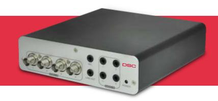
The DSCe150-E004 Video Server transforms 4 analog video inputs to high quality IP video streams. Advanced software captures and encodes analog video and audio signals, and compresses the data to leading-edge H.264 / MJPEG dual Codec. The result is high quality video with significant savings in bandwidth and storage.
